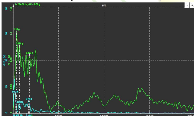
Figure 3: Impact Hammer at Middle position of Beam 2 (120mm from free end) at crack depth 0.1mm
