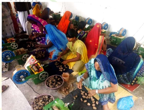
Fig.3: Women reeling silk through motorized reeling machine
